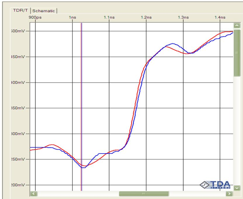
**Figure 13: TDR of the odd reflected TDR pulse with the simulation results. The correspondence establishes the integrity of the measure-based method of determining package impact on system crosstalk.**
